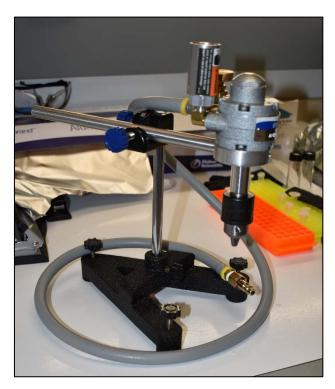
Fisherbrand<sup>™</sup> Air-Powered Analog Overhead Stirrers Used with Ace Oil Bath: Variable speed and explosion-proof stirrers ideal for safely mixing all types of solvents, lacquers and volatile chemicals without the possibility of spark ignition.
